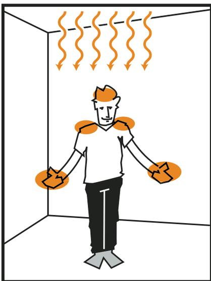
Radiant heat felt from above.
